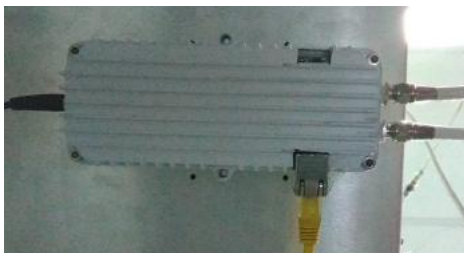
Figure 1: Xemulator mounted on RF chamber
