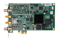
When equipped with the optional NOVELSAT NS4 waveform, the NS10C/NS20C cards support high data rates of up to 425Mbps using 80Msps, enabling transmission of a single carrier over an entire 84MHz transponder. NOVELSAT NS4 delivers satellite bandwidth savings of up to 45% compared with DVB-S2 and 21% vs. DVB-S2X. The NS20C also packs ground breaking signal processing methods such as an adaptive equalizer and error correction techniques that enable the receiver to be more resilient to impairments.
