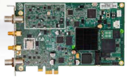
NovelSat NS10C Satellite Modulator Card
