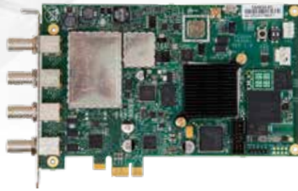
NovelSat NS20C Satellite Demodulator Card
