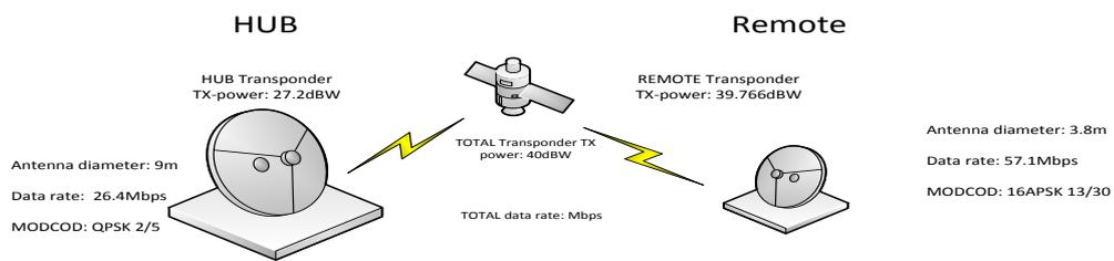
**Asymmetric Data rate, Asymmetrical antenna diameters**
