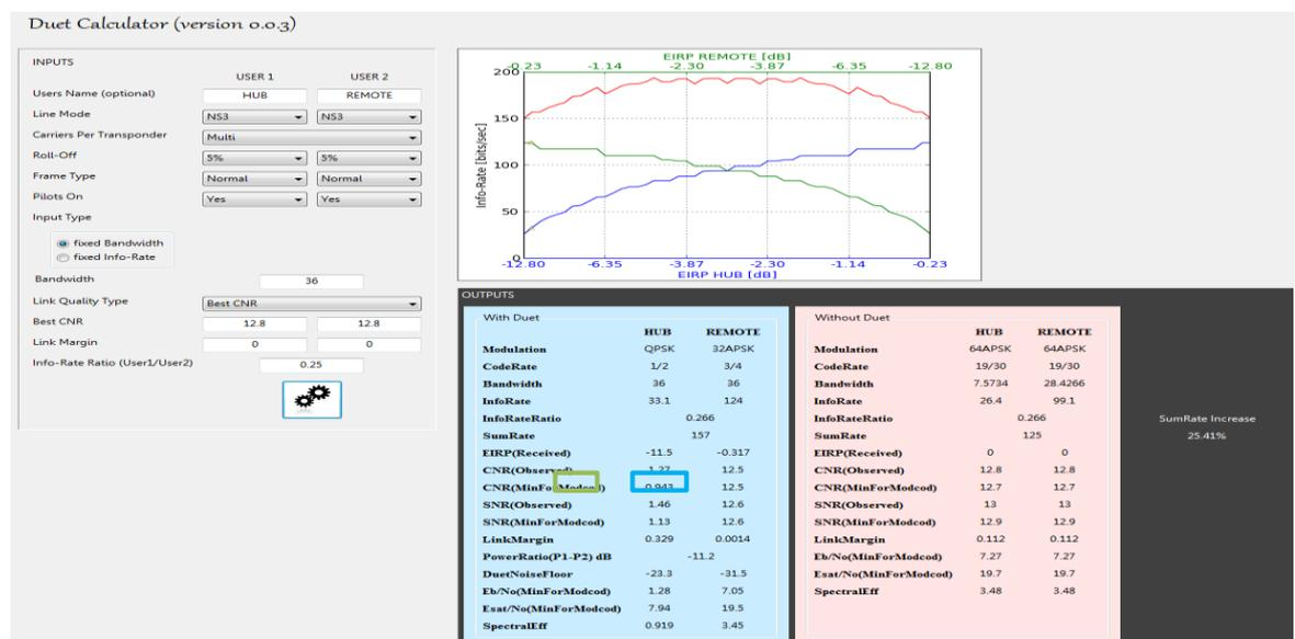
NovelSat DUET calculator for asymmetric data rate, symmetrical antenna diameters
