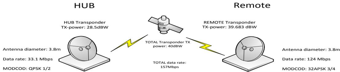
**Asymmetric Data rate, Symmetrical antenna diameters**
