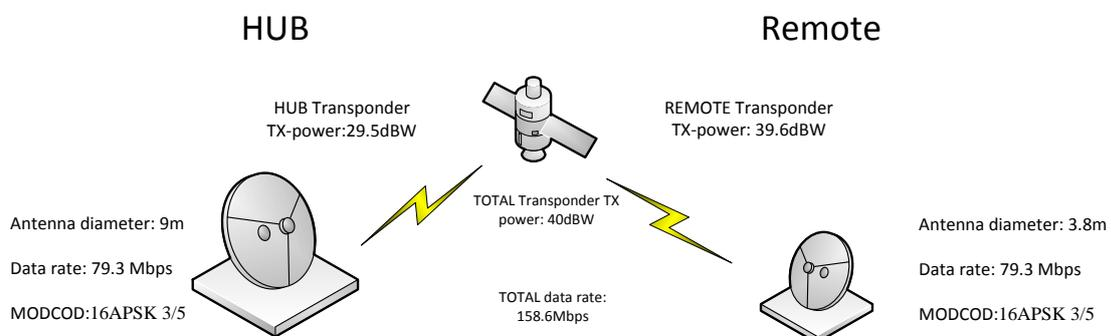
**Symmetric Data rate, Asymmetrical antenna diameters**
